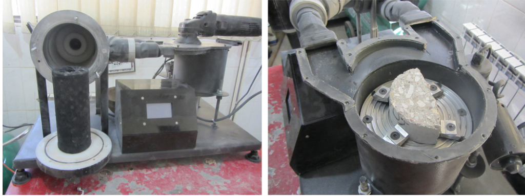
Figure 4. The device used to obtain concrete powder samples at different depths from the exposure surface (Samimi et al. , 2017)
