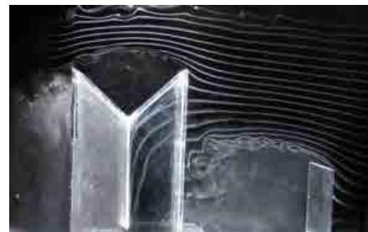
Fig. 10 Visualized flow pattern around and inside the two-sided wind-catcher with upstream structure ( h=0.5H & X=0.75H )
