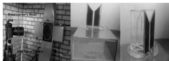
Fig. 8 Experimental setup and wind-catcher model
