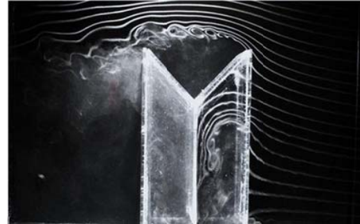
Fig. 9 Visualized flow pattern around and inside the isolated two-sided wind-catcher
